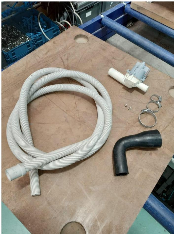
All necessary spare parts to install the drainage pump.
