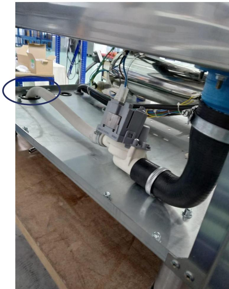
Drain hose is a white and longest one. As explained earlier, the right side of the white hose should be connected to the drain pump and the left (other) side of the hose should be extracted to the outside from the biggest left hole in the body as in the picture.
