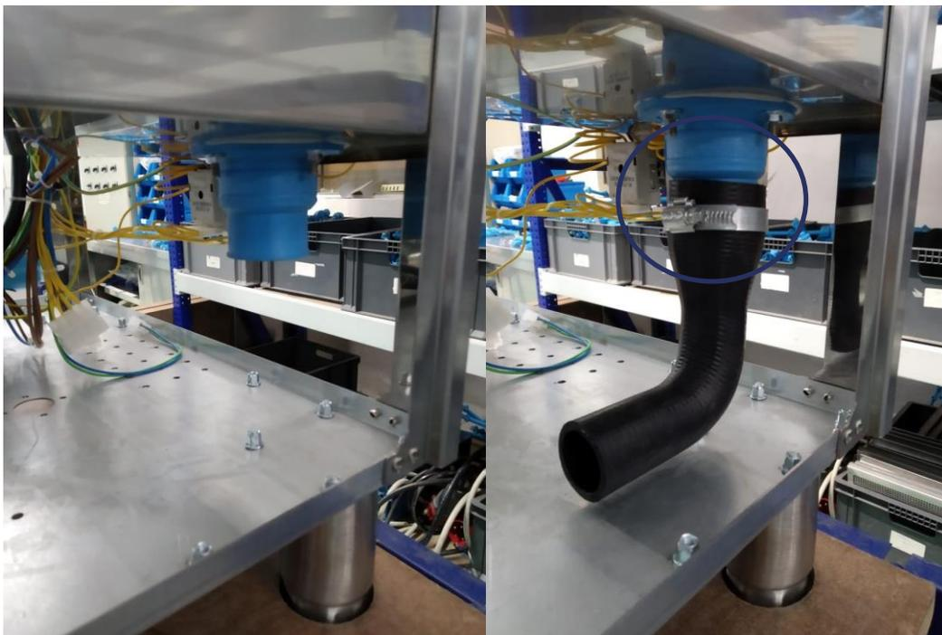
This black hose is part of Drain Pump, so after removing the gray hose, you have to put instead black hose and with the help of hose clamp you have to tight it to the blue plastic which comes out of the machine.
