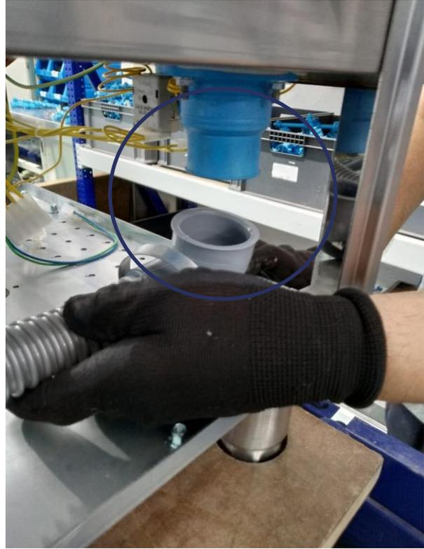
This is the hose for Hood Type Dishwasher without Drain Pump. So, if you want to replace it with Drain Pump, you should remove the gray hose first.
