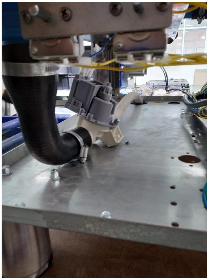
Note: Please make the connections in correct way and tight all hose clamps properly to prevent any water leakage.
