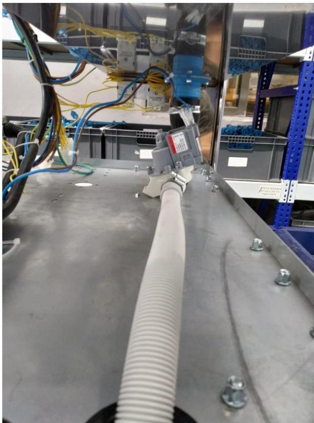
All the cables and hoses are connected to the drain pump.
