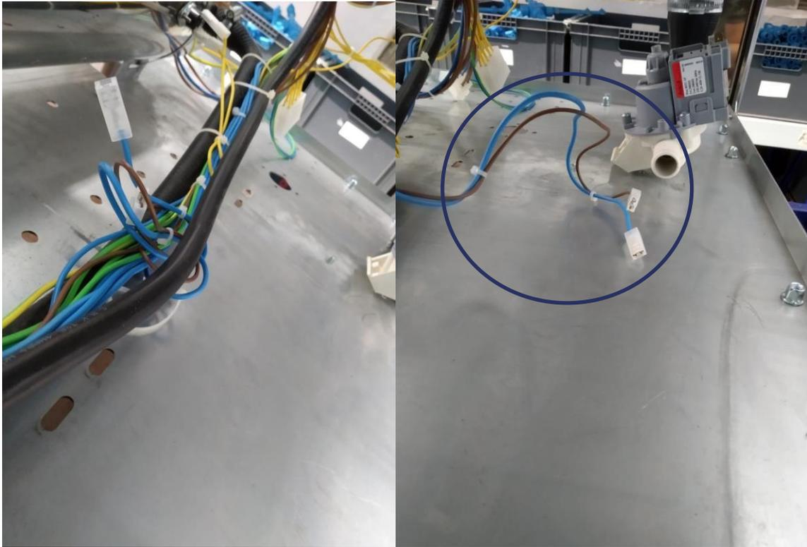
You will find the cable group and there are two cables, blue and brown which have a white connection head or on the cables it is written either Drain Pump or Drenaj Pompası in Turkish. Extend the blue and brown cable from its place to connect the drain pump.
