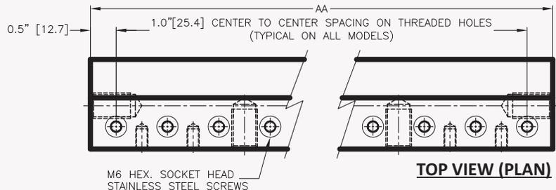
M6 THREADED THRU HOLES CAN BE USED AS ALTERNATIVE MOUNTING HOLES
