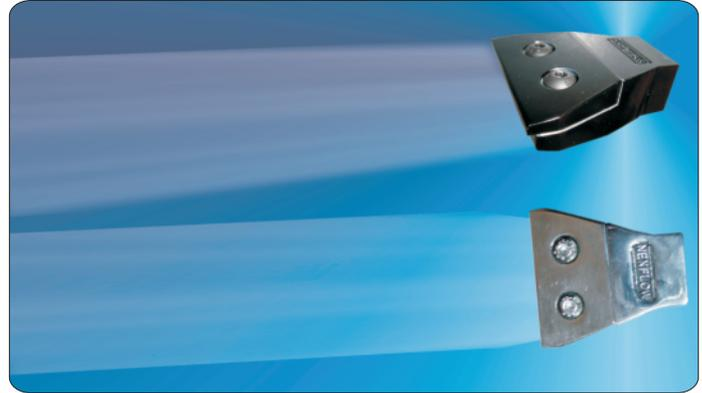
The **Nex Flow™ Air Edger™ Flat Jet** is available with various size “gaps” all set by a flat shim. Three standard shim sizes are available - .004” (.10 mm), .008” (.2mm) and .020” (.51 mm). One, two or more shims can be “stacked” for a larger gap and greater force.
