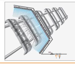
Three 24" X-Stream<sup>™</sup> Air Blade<sup>™</sup> Ionizers Blow off dust from Automotive Bumpers prior to painting. The NEX FLOW™ PLCFC controls the air on and off as required minimizing air consumption. In this case the static bars were "daisy-chained" together minimizing extraneous cable and reducing the number of power supplies needed.
