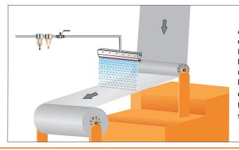
A Model 16118X removes static from extruded rubber web on a rewind. Previously the static charge was so high that any spark would cause the rubber to burn which regularly happens the 'extra strong' VS Bar combined with the X-stream<sup>™</sup> Air Blade<sup>™</sup> eliminated this unsafe situation.
