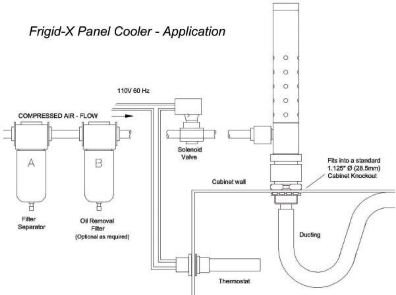
5. Close off any vents or other openings that may draw in ambient air, especially in warm or hot high humidity environments. This entrained air can condense inside the control enclosure much like water that forms on the outside of an ice-filled drinking glass on a summer day. Relocate any external fans inside the enclosure to help circulate the internal cooled air.
