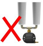
Avoid water pockets when installing the drain pipe, this will create an air lock.
