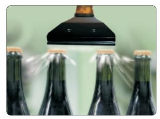
Air Edger<sup>™</sup> Flat Jet with .008" gap setting blows water from under the caps on a bottling line moving at high speed
