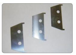
The Air Edger<sup>™</sup> Flat Jet Nozzle air gap is set by one or more shims. There are three basic shim sizes - .004" (.1 mm), .008" (.2 mm) and .020" (.5 mm). Shims may be stacked for larger gaps and for sizes in between the shim standard sizes offered. Shims available in both 304 stainless steel & 316L stainless (for the stainless **Air Edger**<sup>™</sup>). The greater the gap the more powerful the force.
