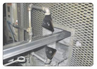
Air Edger<sup>™</sup> Flat Jet with .020" gap setting provides a powerful force to blow of dirt and debris in an extrusion line
