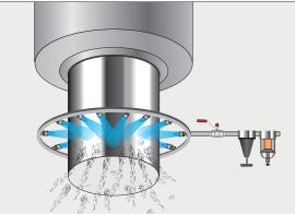
Model 47003 Nozzles are mounted along the circumference of a one meter diameter piston rod to blow off debris from its surface. The Nozzles are operated only when piston rod retracts in to the cylinder.
