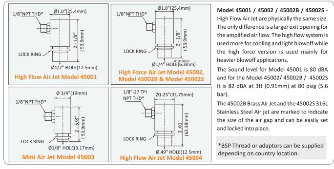
Air Jets perform similar to Adjustable Air Amplifiers - with the same lock ring and methodology. **Nex Flow™** Air Jets are adjustable and come with a lock ring to fix the gap.
