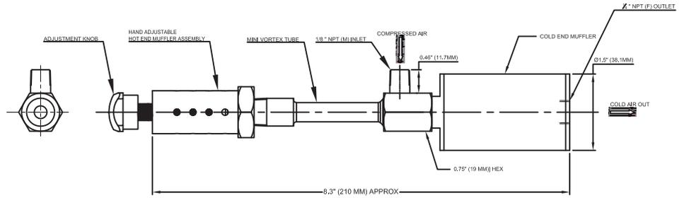
**SMALL VORTEX TUBE WITH GENERATOR, HAND ADJUSTABLE HOT END MUFFLER ASSEMBLY + COLD MUFFLER + SINGLE POINT HOSE KIT**
