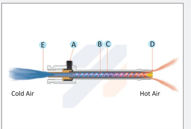
**Due to space limitation & the need to eliminate water cooling the camera, a Model 50025H Vortex Tube was used to cool a camera housing.**
