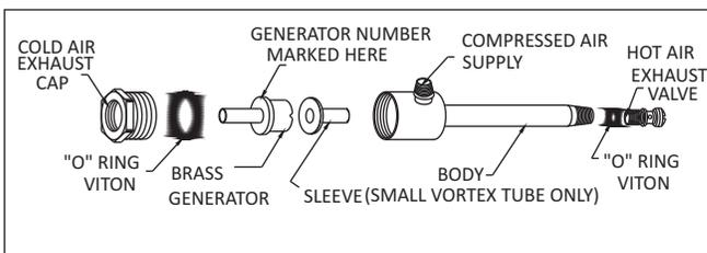
**CONTROLLING THE FLOW RATE AND TEMPERATURE IN THE FRIGID-X™ VORTEX TUBE**
