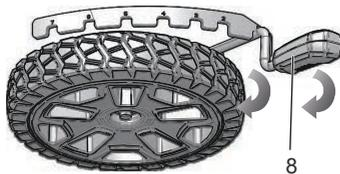
1. Pull the height adjustment lever (8) rearward to increase the cutting height.
