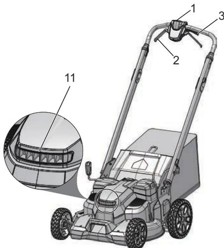
1. When the mower is ready to start, you may grab the start handle (2) or the self-propel lever (3) to turn on the LED headlight (11).
