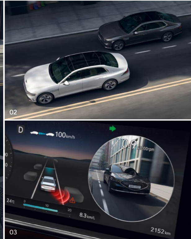
03. Blind-Spot View Monitor (BVM) system _ When the turn signals are activated, video images of the respective side/rear view of the vehicle appear on the center cluster.
