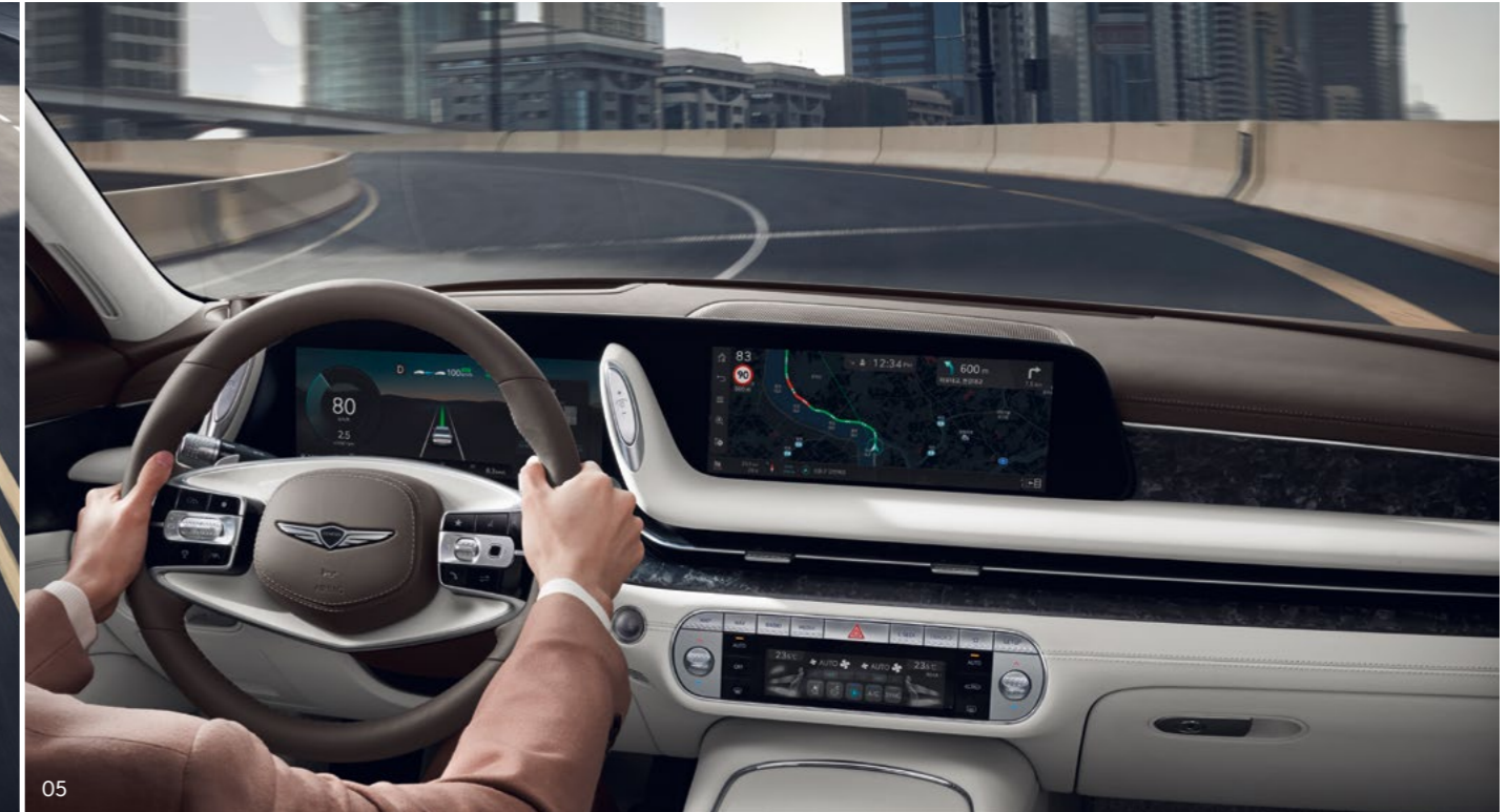
05. Navigation-based Smart Cruise Control (NSCC) system _ This system automatically slows down the vehicle upon entering a limited speed zone area or a curved section, returning to its previous set speed afterwards. It also reduces the speed when entering/exiting a highway, assisting in safe driving.
