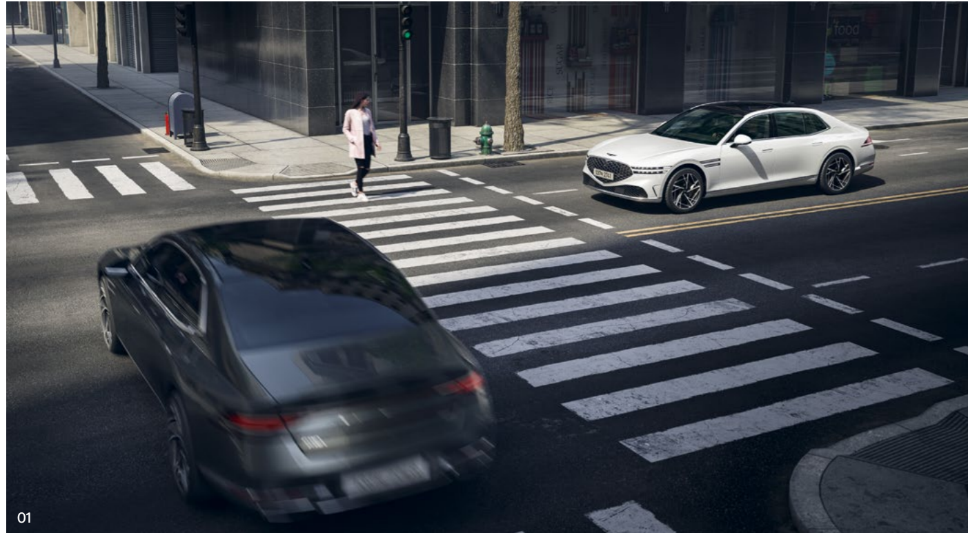
01. Forward Collision-Avoidance Assist (FCA) system _ When a collision risk with a vehicle/pedestrian/bicycle ahead is detected, this system warns the driver and, if necessary, helps to control the brake to avoid a collision. When there is a collision risk with vehicles approaching from left/right sides of an intersection, it automatically assists in braking. It also assists in steering if there is a collision risk when changing lanes.
