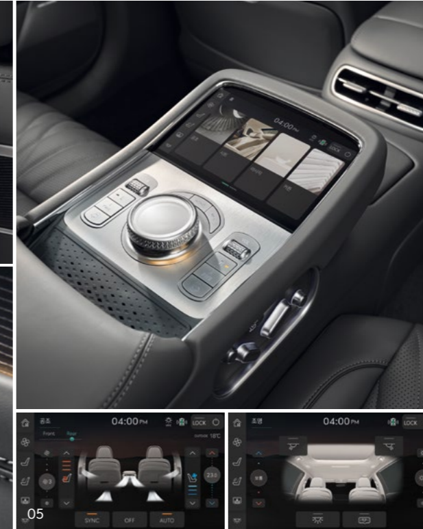
05. 8" armrest touch screen (ATS) _ Rear seat passengers can control climate control modes, seat positioning, massage modes, curtain settings and lighting via a touch screen monitor on the armrest. The monitor is easy-to-use, with graphics and animations identical to real images of the vehicle.
