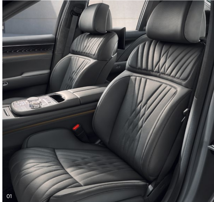
01. ERGO relaxing seat _ The 10 air cells on the seatback and two air cells on the cushion provide four massage modes, including a whole body massage. The seats are also linked to vehicle speed, the rear seat's one-step mode, and the mood curator system to ensure optimal seating at all times.
