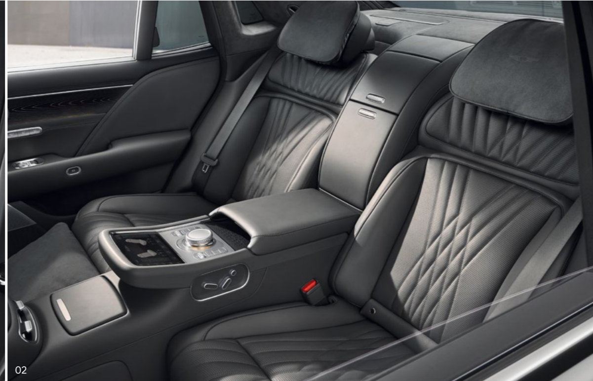
02. First class VIP seat _ The reclining and sliding functions of the VIP seat-which can be adjusted independently from the other rear seat-are linked, while the reclining function offers ideal tilting options. The connected-type leg rest and foot rest also provide maximum comfort for long drives.
