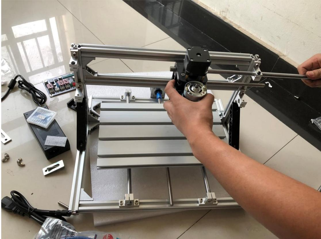
7. The slide bar is then eased out of one side enough to allow the z axis / motor assembly to be inserted.
