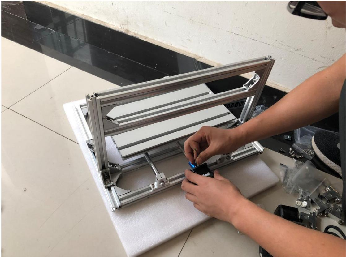
5. The carriage assembly is then moved over to the left hand side and the support bracket tightened up.
