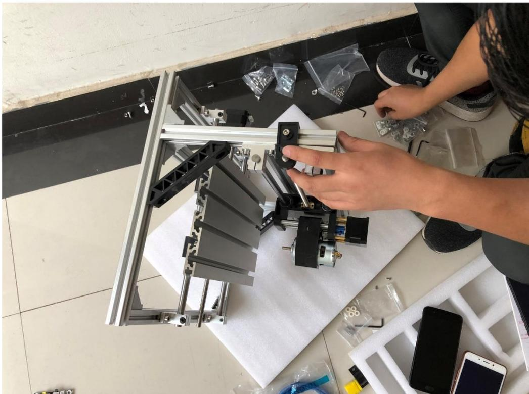
11. Slide to both ends to ensure free movement, then with the assembly at the left side tighten the Left bottom bracket, and finally move to the right and tighten the bottom right bracket.
