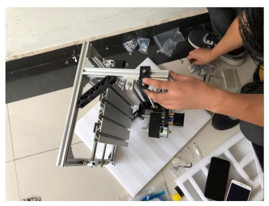
11.Slide to both ends to ensure free movement, then with the assembly at the left side tighten the Left bottom bracket, and finally move to the right and tighten the bottom right bracket.
