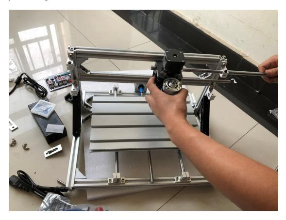
7. The slide bar is then eased out of one side enough to allow the z axis / motor assembly to be inserted.
