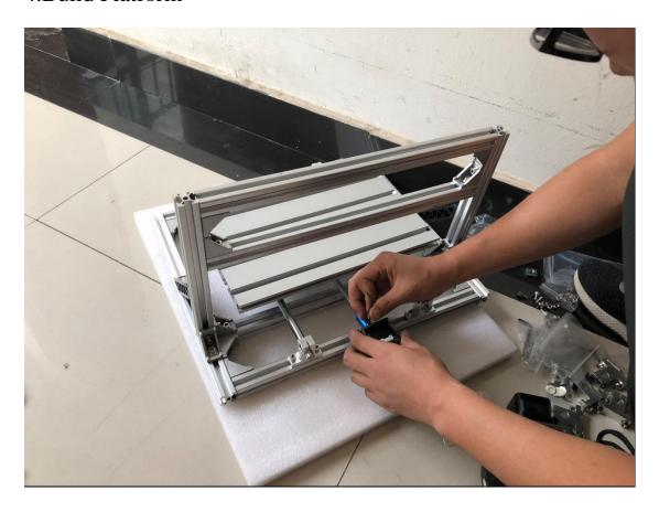
5. The carriage assembly is then moved over to the left hand side and the support bracket tightened up.
