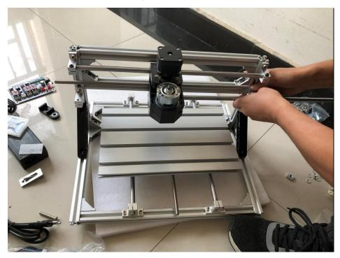
8. The carriage assembly is then move3d over the the right hand side and the motor is aligned with the coupling and tightened in place.
