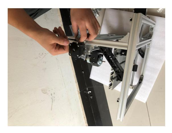
10. Now move the assembly to the left and tighten the top left bracket.
