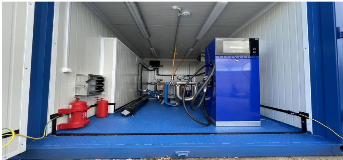
Figure 3. Drilling rig, steam generator set
