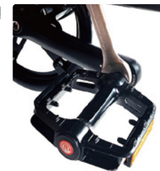
Tighten the left pedal "L" counter clockwise
