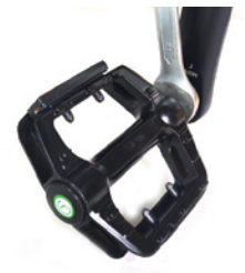
Tighten the right pedal "R" clockwise
