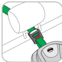
Now take the top tether (**TT**) and guide it along under the headrest of the vehicle to the appropriate top tether anchorage point of the vehicle.
