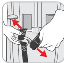
Afterwards you can release the harness belts (G2) and the shoulder pad belts (SG) from the adjustment unit and pull out both belt ends through the shoulder belt lead-through (G1).
