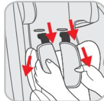
In order to remove the crotch strap, push the belt, together with the metal plate, out of the seat part from bottom to top
