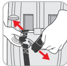
Loosen the belt ends of the harness belts (**GZ**) on the back side of the seat part (**ST**) from the belt anchor (**R**).
