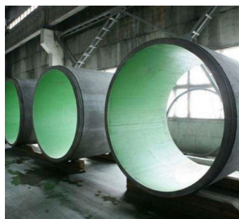
CONCRETE PIPES LINED WITH POLYMER SHEET
