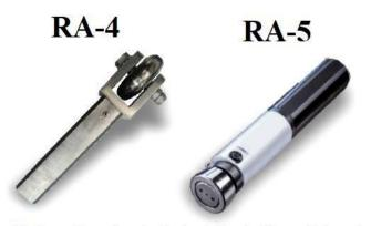
RA-5 one-roller universal roller burnishing tool for machining external surfaces, faces and holes. Minimal machining hole size Ø 34 mm. Shank Ø 35 mm. Maximal machining depth L 200 mm. Workpiece hardness up to 40 HRC.
