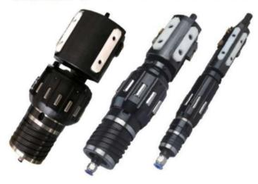
Two-stage combined skivving and rolling tools with the movable head. These tools are used for internal finishing of cylinders and tubes. The tool rolls out any irregularities such as wavinesswhich can occur in the production of hydraulic cylinders.
