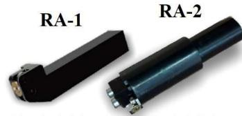
Tool for surface hardening and roller burnishing of cylindrical parts made of regular and hard-to-machine materials (titanium, nickel alloys, inconel). Shank size 20x20,25x25, Ø 32, Ø 40
