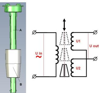
By applying an alternating current to the centre coil (**U** in) an output voltage (**U** out) is created between the two outer coils. This output voltage depends on the position of the float. See the schematic above.
