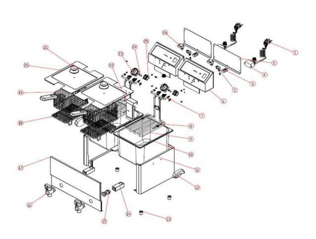
2.cover of electric box 1.Power line **5.**Contact switch 4.relay 7.hanging 8.temperature probe 10.oil pot 11.frame **13.feet** 14.square tube 16.oil tap 17.face plate 19. frying basket 20.cover of oil pot 22.protect board 23.thermosistor 25.mains switch 26. temperature limiter 3.connector
