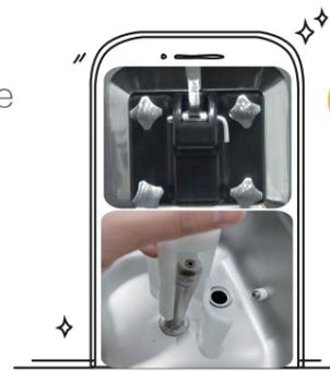
09 Install the handle,fixed with the fixed pin,put the agitator blade
