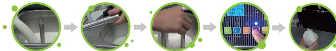
01 Pull the material 02 Close air tube 03 Insert air tube 04 Press AUTO 05 Making ice cream
