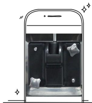
08 Install the nut,ensure the nut is tight ,the discharge door is sealed well
