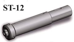
ST-12 diamond burnishing tool for holes is used for smoothing out through holes Finishing is done in 2 passes only. The length of the hole is not limited. It is possible to produce tools with longer length of treatment (up to 1000 mm and more) is possible. Versions for machining diameters: Φ30, and larger.Internal coolant supply
