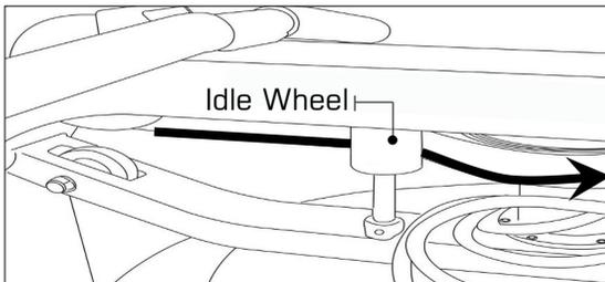
Next, thread the Belt around the Idle Wheel as shown. Once around the Idle Wheel, attach the Rower Belt to the Belt/Bungee Pulley. There is an obvious "lip" at the attachment point.
