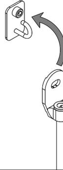
**!** Do not cut Bungee tie wrap before Bungee cord is attached to rear of the Rower as shown here.
