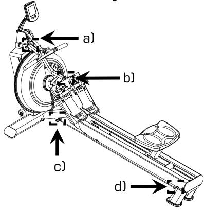
a) Carefully lower the Rower to its normal operating position to complete assembly with S-bend installation and Frame Tension Cable.
