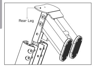
b) Install all M10x47.5mm Bolts[15] and M10 Washers [23] first from the outside to hold the Rear Leg [7] in position.
