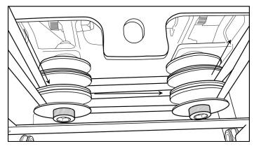
Middle right Pulley to upper right Pulley.
