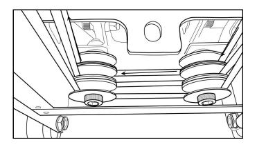
12. Upper left rear Pulley to tie off point. Finish the Bungee rewrap by tying off the Bungee. You may elect to not use a tie wrap as the metal tab is designed as a stand alone attachment point. Thread the Bungee through to desired tension and thread the Bungee end through the upper hole as shown.
