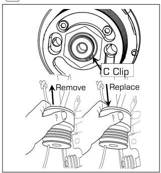
6. Move the Rowing Handle from the S-Bend to a point where it is resting on top of the Tank. This helps line up the Bungee Cord hole for easier removal/replacement. Detach Bungee Cord from lower rear attachment point.
