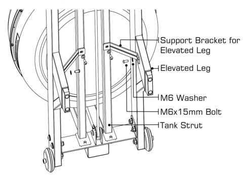
Using 4x M6x15mm Bolt[12], 4x M6 Washer[11], attach the 2x Support Bracket for Elevated Leg[8] to the Rear Brace and Elevated Leg.
