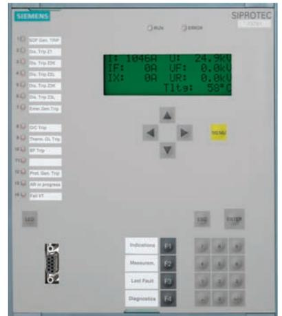
Operator panel of Siprotec 7ST61 protection relay
