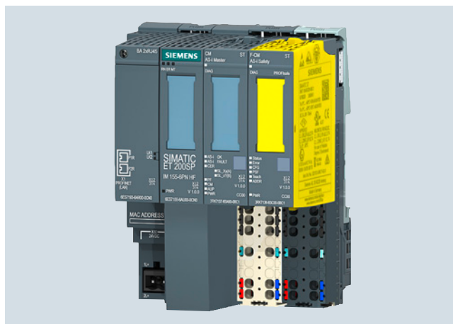
Combination of an ET 200SP interface module, CM AS-i Master ST and F-CM AS-i Safety ST
