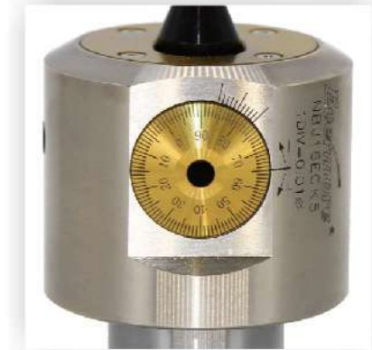
刻度盤最小刻度每小格0.01mm The smallest graduation 0.01mm
