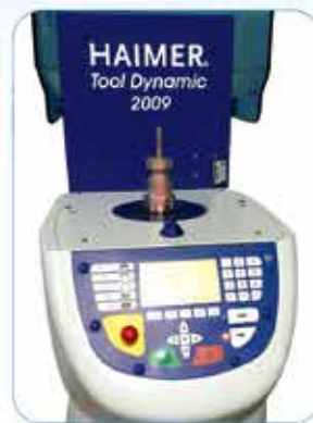
刀柄动平衡检测 accuracy dynamic balance
