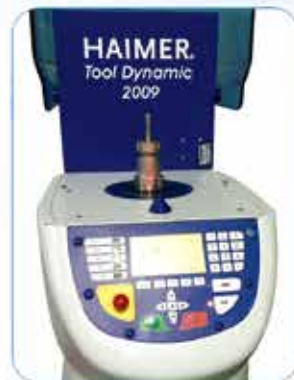
刀柄动平衡检测 Accuracy dynamic balance
