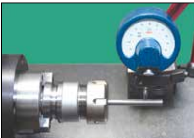
同轴度 (综合精度) 检测 Inspection of coaxial degree (overall accuracy)
