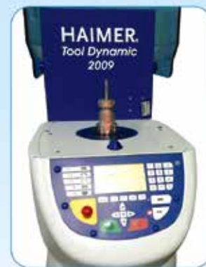
刀柄动平衡检测 accuracy dynamic balance
