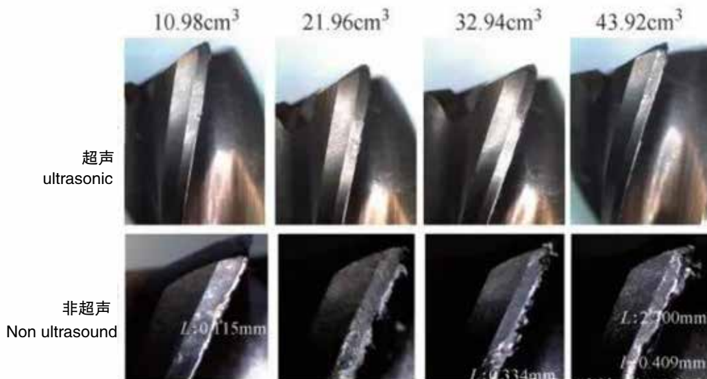
超声与非超声加工钛合金刀具磨损对比 Comparison of wear between ultrasonic and non ultrasonic titanium alloy cutting tools
