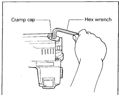
Rest the tool on the table with the bit end pointing upwards. This will allow the old grease to collect inside the crank housing. Wipe out the old grease inside and replace with a fresh grease (60 g). Use only Makita genuine hammer grease (optional accessory). Filling with more than the specified amount of grease (approx. 60 g) can cause faulty hammering action or machine failure. Fill only with the specified amount of grease. Reinstall the crank cap and tighten with the hex wrench.
