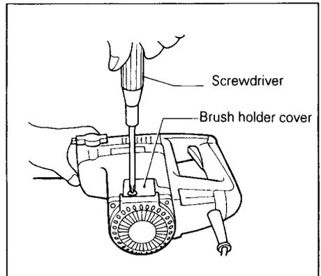
Use a screwdriver to remove the brush holder caps. Take out the worn carbon brushes, insert the new ones and secure the brush holder caps.
