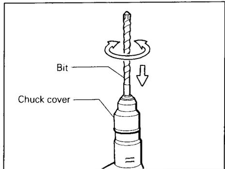
If the bit cannot be pushed in, remove the bit. Pull the chuck cover down a couple of times. Then insert the bit again. Turn the bit and push it in until it engages.
