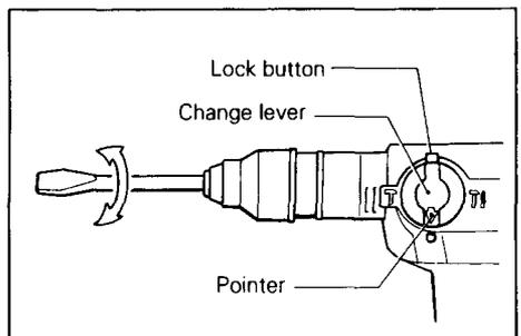
Depress the lock button and rotate the change lever so that the pointer points to the
