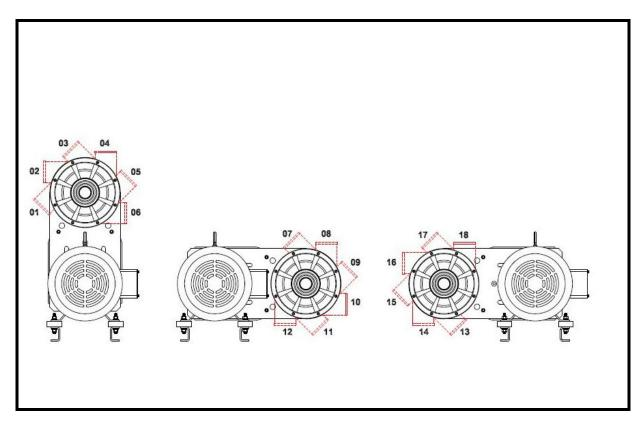
For Blowers **Rotations 07-12**, Kit P/N 15463 (Kit-Extension Filter Silencer) is needed to connect the filter silencer due to the interference with the Motor Junction Box
