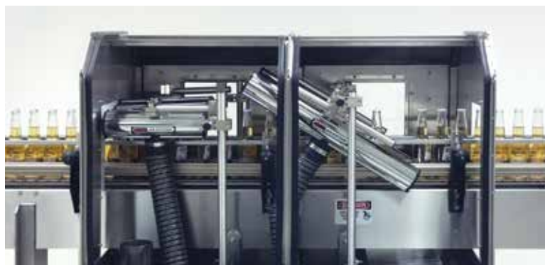
Air Knives are sized and positioned to suit the application
