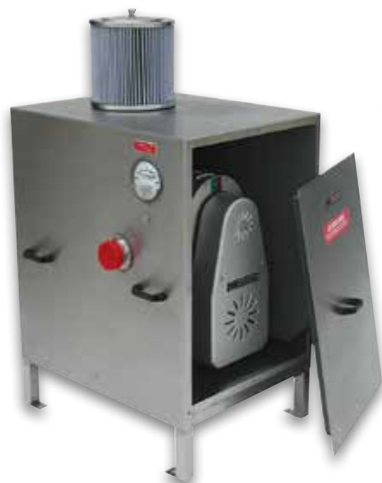
Blower/Motor Enclosures reduce noise levels to 75 dB. 10 micron pre-filters protect the system from airborne contaminants
