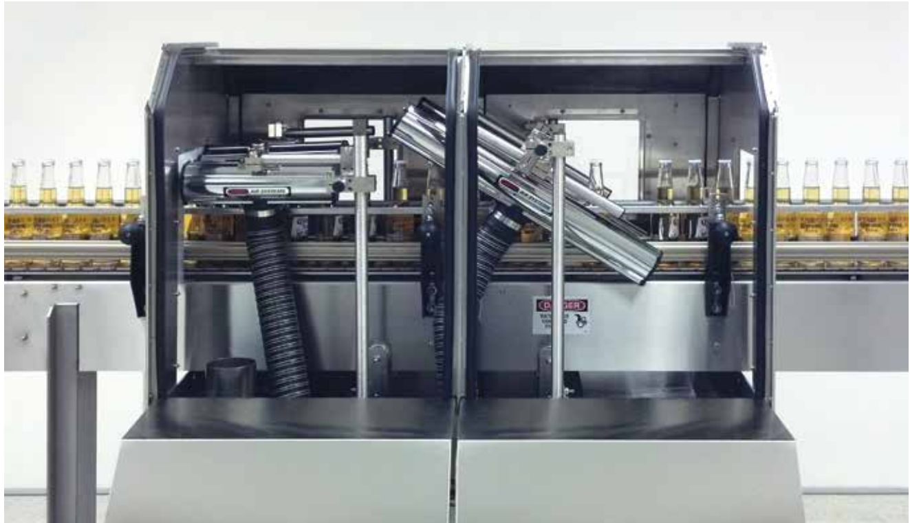
Covers removed to show Air Knife orientation in tunnel interior
