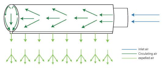
Republic air knives incorporate a tear drop design to minimize the internal turbulence of air entering the knife while projecting it in a highly controlled manner through the discharge. As the air enters the knife, the lack of sharp edges within the knife minimizes pressure loss and turbulence while the air moves along the walls and is concentrated at the discharge.
