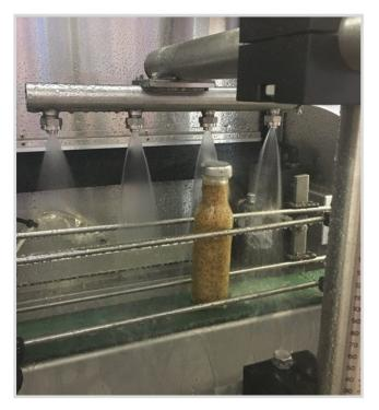
Built to wash cans, bottles and jars, the **PowerWash** uses micro-nozzles to provide precise and efficient rinsing across the entire surface of the container, whilst minimising water consumption.
