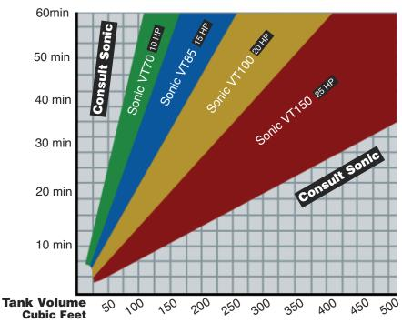
The Sonic DRY-IN-PLACE<sup>TM</sup> System models shown in the data above represent the four most common units selected for the total volume of tank circuits listed. The actual model and Hp required for every application are determined by Sonic.
