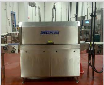
Including an open mesh conveyor, hold-down belt and dedicated gusset drying, the **Pouch Dryer** is suitable for all types of flexible packaging, including:
