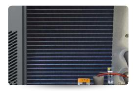
All models in the **TREF CW** range feature heat exchange coils with **hydrophilic coating**. This special coating - together with adequate adjustment of air through-flow speeds - helps condensate collection during the dehumidification process, avoiding dripping on the inside and outside of the unit.
