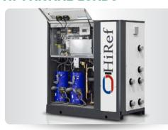
Accurate selection of the components allows high efficiency to be obtained at partial loads; this is thanks above all to the use of scroll compressors and to the use of electronically controlled electric expansion valves (one for each circuit), optimised to track refrigerant load trends in all conditions of use. The plate heat exchanger also ensures low water/refrigerant approaches during operation, all to the advantage of heat exchange efficiency.
