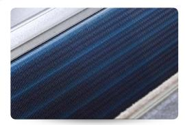
All models in the monobloc interior range feature **evaporating coils with hydrophilic coating**. This special coating - together with adequate adjustment of air through-flow speeds - helps condensate collection during the dehumidification process, avoiding dripping on the inside and outside of the unit.
