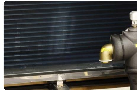
All models in the **TREF Free-Cooling** range feature heat exchange coils with hydrophilic coating. This special coating - together with an adequate adjustment of air through-flow speeds - helps condensate collection during the dehumidification process, avoiding dripping on the inside and outside of the unit.
